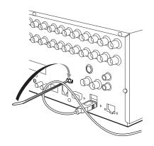
step3. Pull the edge of the cable clamping band until it stops.
